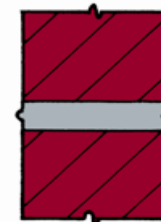
Beaded Moderate Weathering
