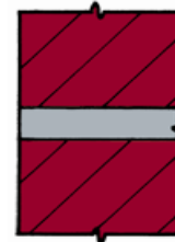
Flush Negligible Weathering
