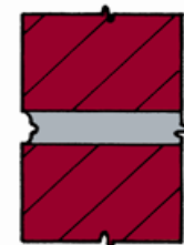
Grapevine Severe Weathering
