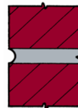
Concave Severe Weathering
