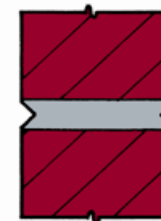
V Severe Weathering
